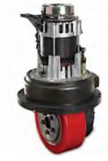
The drive tire is cantilever mounted on the drive unit, and can be removed with 5 bolts to change out in just minutes.
