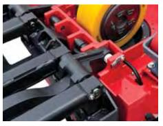
Fork-height adjustment is simplified by using eccentric pins at fork heel for improved pallet entry and exit.
